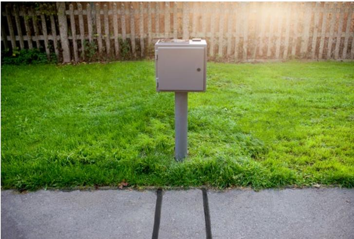
RidePod™ BP permanently installed bike monitoring system on a shared path.
