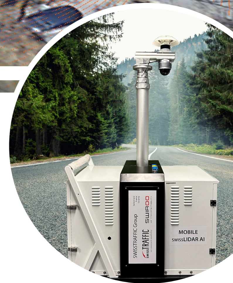
Mobile LiDAR version for short-term deployments and greater flexibility.
