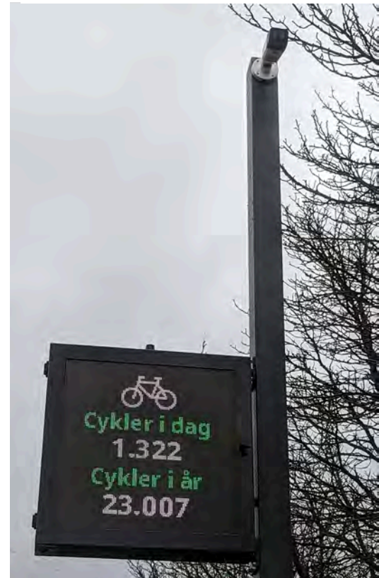
AI Display board with external AI camera (internal solution available).
