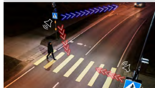
Real-time automatic detection of right-of-way violations at pedestrian crossings and warning of road users.
