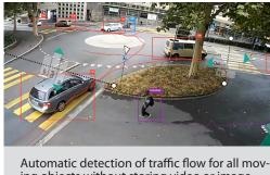
Automatic detection of traffic flow for all moving objects without storing video or image data.
