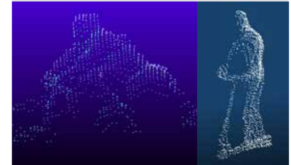
A cloud of points indicating a bicycle and an e-Scooter. The sensor software is able to distinguish cyclists, e-scooters and pedestrians.
