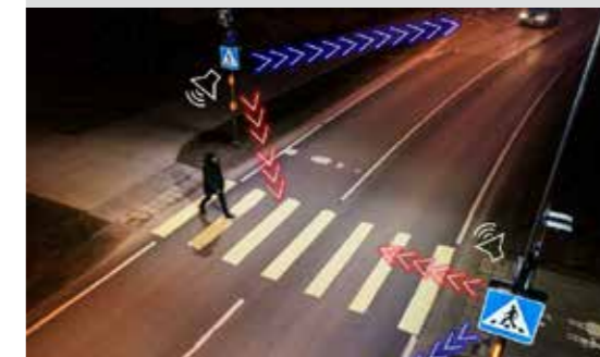
Automatic detection of failures to give way at pedestrian crossings in real-time and warnings for road users.
