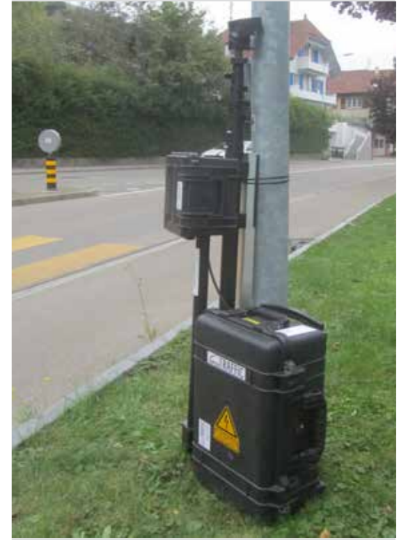
Mobile camera system with integrated AI analysis software for real-time evaluations and presentation on a proprietary dashboard.
