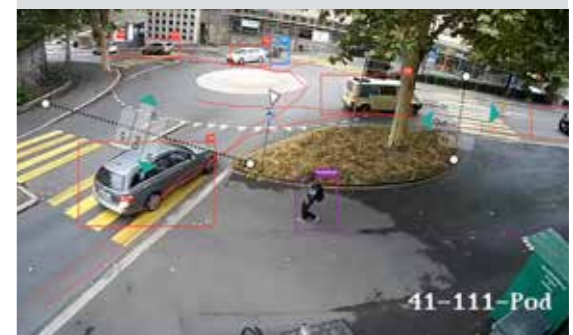
Automatic detection of traffic flow for all moving objects without storing video or image data.
